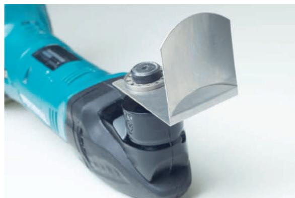
**VB-001** Vibra-Blade is the ultimate tool for vibrating concrete. Use along the edge forms to remove nearly all trapped air which causes unwanted “bug holes” in the countertop edge. This tool attaches to nearly all brands of Multi-Purpose Oscillating Tools. Note: It will not work with Dremel Quick-Change system. Tool Sold Separately.
